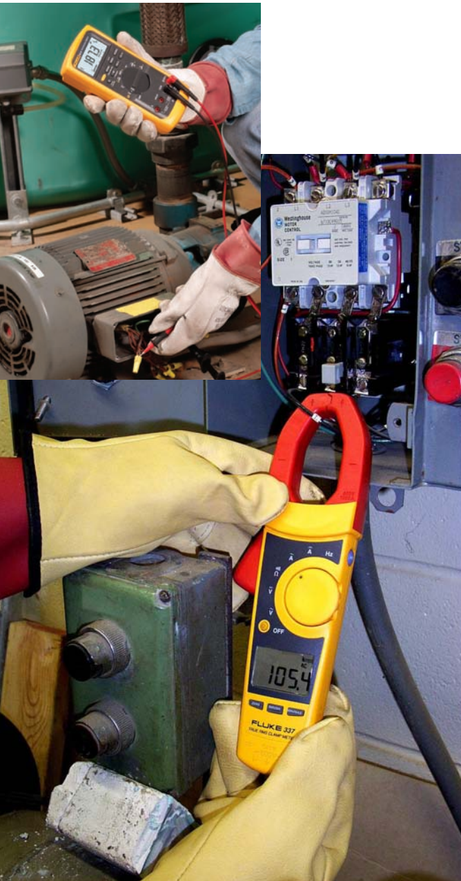
A clamp meter with an inrush function can greatly reduce the time needed to troubleshoot a motor problem.
