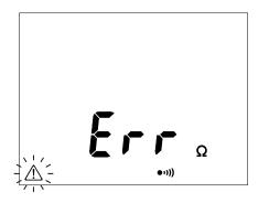
If, during a continuity, resistance, or capacitance measurement, the instrument detects an external voltage in excess of 15 V (AC or DC), it interrupts the measurement and displays the screen shown opposite.
