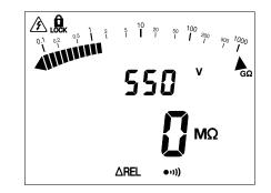
If the measured value is less than the stored value, the display becomes negative.
