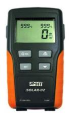
With SOLAR-02 remote unit the irradiance and temperature measured values are shown at display also in independent mode (ideal solution during a pre-test on installation) besides test/recording with SOLAR I-V
