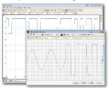
Every model includes a built-in DC to 20 MHz function generator with sine, square, triangle and DC waveforms. D models add a built-in 12-bit, 200 MS/s arbitrary waveform generator. You can import arbitrary waveforms from data files or create and modify them using the built-in graphical AWG editor.
