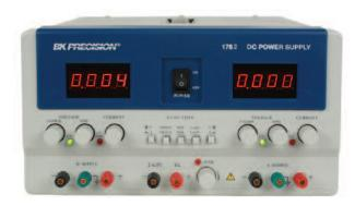
Model 1762 Triple Output DC Power Supply delivers 0-60 V/0-2 A on 2 outputs and 4-6.5 V/4 A on 1 output. The 4 digit LED display offers 10mV and 1mA resolution, providing the capability to set voltage and current values more accurately and precisely compared to 3 digit displays found in most comparable power supplies. The power supply is fully overload protected and comes with a two year warranty.
