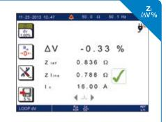
is sufficient for the installation. The result of this  $\Delta V$  measurement is displayed in %; if the value is greater than 5 % or a programmed value, the sizes of the cables for the installation must be recalculated.
