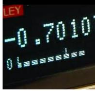
The Model 2002's unique one-phase four-wire ohms measurement capability makes it a good solution for high speed production testing of precision resistors. Two high and two low limits can be tied to the status of any of four protected digital outputs, so the Model 2002 can sort or grade the resistors automatically after testing. For QA tests on small samples, the front panel bar graph display makes it easy to determine the tolerances of individual resistors.
