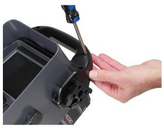
2. Pull the two halves of the docking handle apart, including the rubber grip insert and both docking joints.
