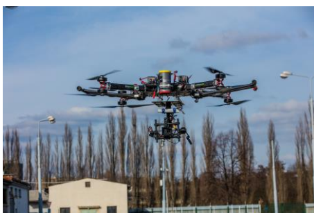
Workswell WIRIS system on the drone
