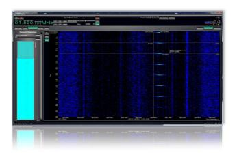
Spectrogram / Waterfall View for the identification of frequency hops, measurements of pulse rate, analysis of time variant spectra and the tuning of a VCO
