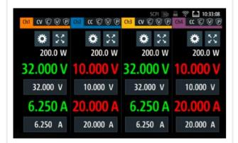
The home screen gives a clear overview of all channels. Each channel can be selected for a more detailed view containing a wide variety of additional information such as statistics and icons indicating the status of set protection levels and special functions.
