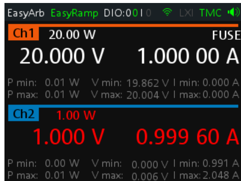
Figure 6-3: Output of Ch2 in CC mode
