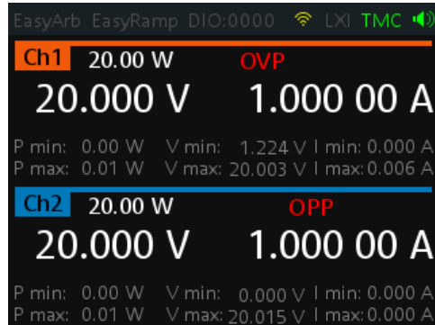
Figure 6-8: Indicator of OVP/OPP when tripped
