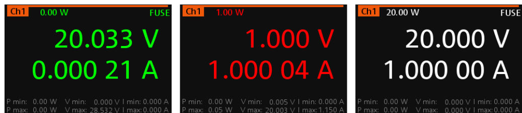
Figure 5-3: Color coding of difference operating conditions
