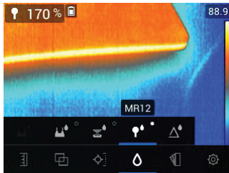
Figure 7.11 Selecting the MR12 (optional Ball Moisture probe) mode
