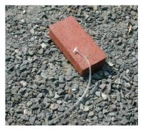
One end of the clear 10 m tubing (for measuring outside pressure) is placed about 10 m from the building. Place a T-piece over this end to prevent disturbances from wind.
