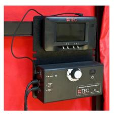
The DG-1000 is mounted on the gauge board using the four magnets on its backside.
