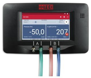
Fig. 4.28: Tube connection at DG-1000
