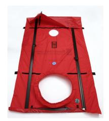
Unfold the BlowerDoor panel on the floor and place the assembled frame on top (with the clamping levers pointing up). The Velcro straps on the panel should also face up.
