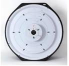
Flow ring D attaches directly to the center of ring B (remove ring C before inserting ring D). The letter D faces upward. When using flow ring D or E, the red tubing for measuring the flow of the fan (fan pressure) connects to ring D.
