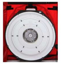
Begin the test with flow rings A, B and C installed.
