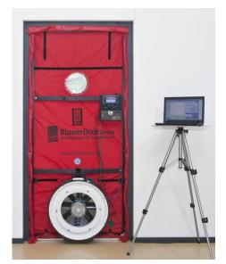
The BlowerDoor system is typically controlled from inside the building. All BlowerDoor equipment (bags, frames, fans, computer, paperwork, cable reel, etc.) is placed in the same room as the testing device.
