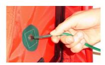
Connect one end of the green tubing to the patch at the bottom right corner of the panel. Outside the building, the clear tubing should have been connected to the same patch.
