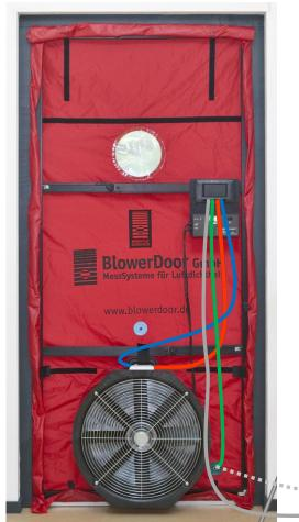
For a **positive pressure test**, the fan is **turned around**. The flow rings point outwards, and air is sucked into the building.
