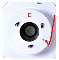
For determining the flow of the fan when using **flow rings D and E**, connect the red tubing to the port on ring D. The blue tubing remains connected to the port marked blue on the fan electrical box.
