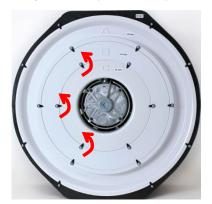
To **change the flow ring**, rotate the ring clips to remove a flow ring. Insert the correct ring face-up (identifying letter facing up and the flow nozzle pointing into the fan) and retighten the fastener clips.
