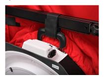
The Velcro strap on the cross bar directly above the opening in the panel holds the fan in place. Pull the strap through the handle on the fan and secure it.
