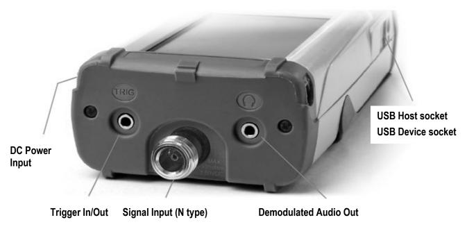
**DC Power Input** 1.3mm power socket mounted on the right hand side of the instrument.
