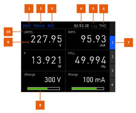
Figure 7-1: Example of screen display in numeric mode
