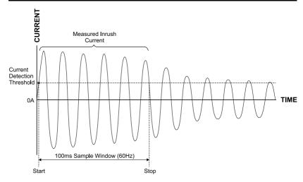
Figure 8.4 Capturing Inrush Current.
