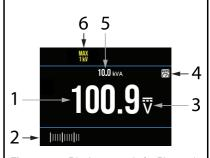
**Figure 8.14** Display example for Photovoltaic power measurements.
