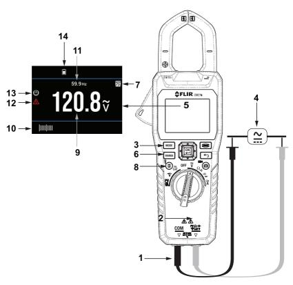
Figure 8.5 AC and DC Voltage Measurement Setup.
