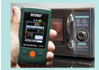
Convenient 3-in-1 EMF meter simultaneously measures and displays Magnetic Field, Electric Field, and Radio Frequency Strength. Ergonomic pocket-sized design with an easy-to-navigate menu. Large vivid color TFT display shows digital readings, bargraphs, and trending graph.
