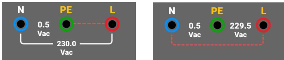
Loop and RCD tests are inhibited and an error message is generated if the input voltage is not between 100 V and 500 V. The UK Loop and RCD tests are inhibited if the L-PE or the L-N terminals are reversed.
